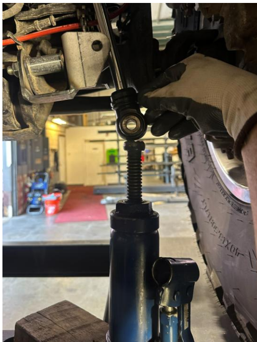
Figure 13: Shock bolt installed, eyelet sits neutral in new outboard mount
