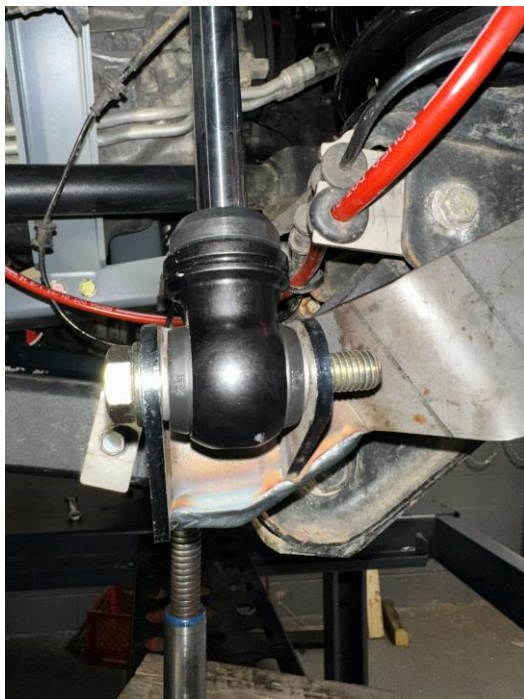
Figure 13: Shock bolt installed, eyelet sits neutral in new outboard mount
