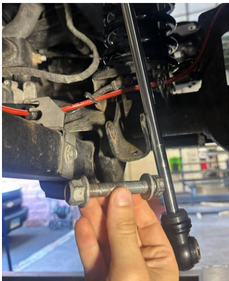
Figure 2: Lower shock bolt removed
