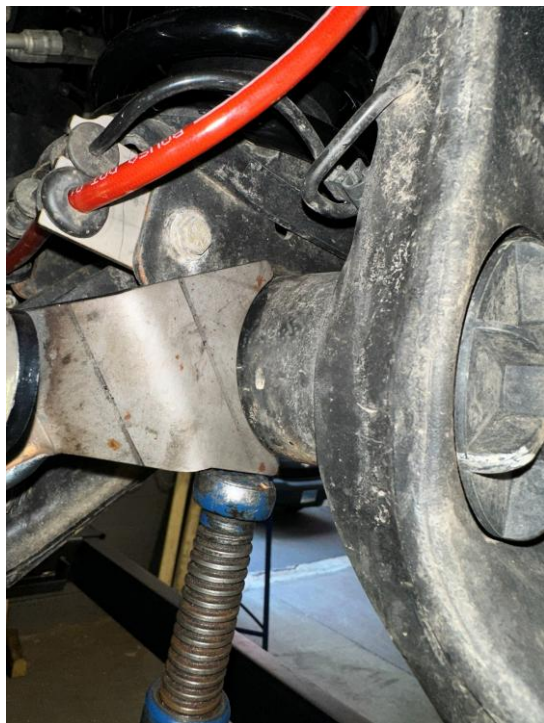
Figure 11: Bottle jack at weld-seam
