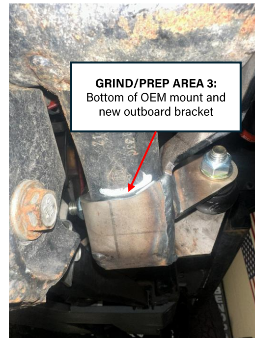
Figure 10: Outside bottom weld area prep
