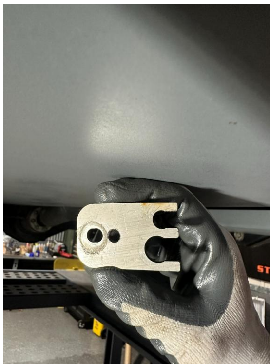
Figure 17: Brake line bracket modification part 2
