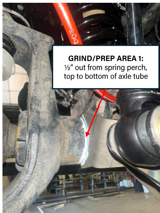
Figure 8: Axle tube weld area prep
