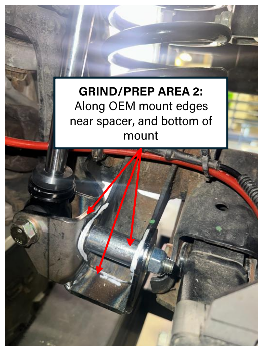
Figure 9: Inner bracket weld area prep
