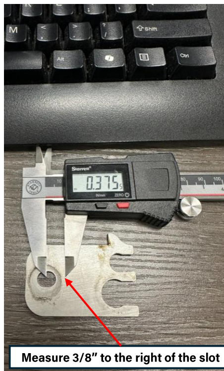
Figure 16: Brake line bracket modification part 1
