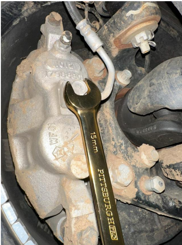
Brake caliper banjo bolt (15mm)
