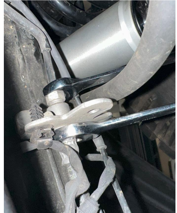
Frame end fitting (16mm and 12mm)
