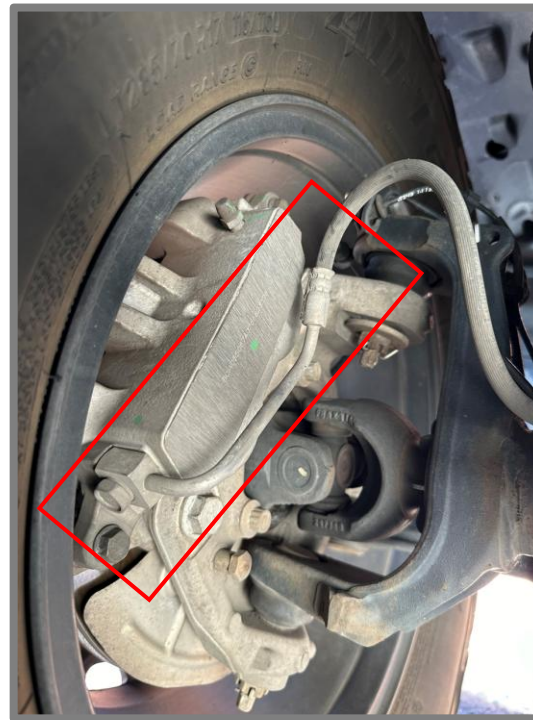
Standard brake caliper Use 1309105
