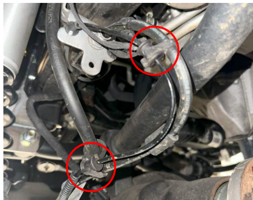
Old brake-line clips to be removed
