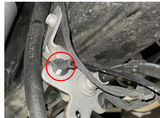
Frame mount ABS cable to be removed
