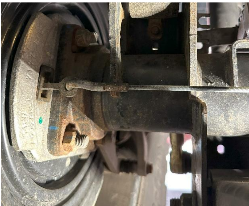
Figure 10: Rear left cable reinstalled in eyelet hook
