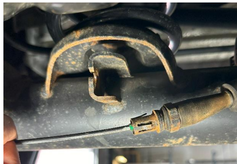
Figure 3: Emergency brake cable housing fully removed from mount
