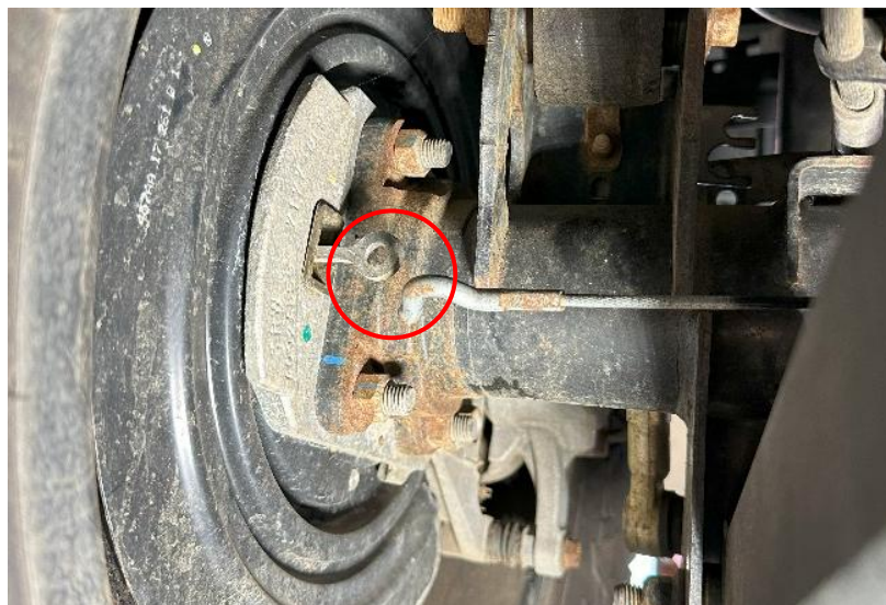
Figure 1: Rear left parking brake cable removed from eyelet
