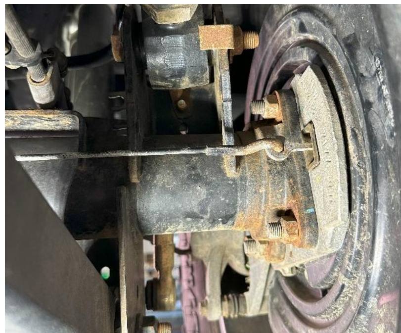
Figure 11: Rear right cable reinstalled in eyelet hook
