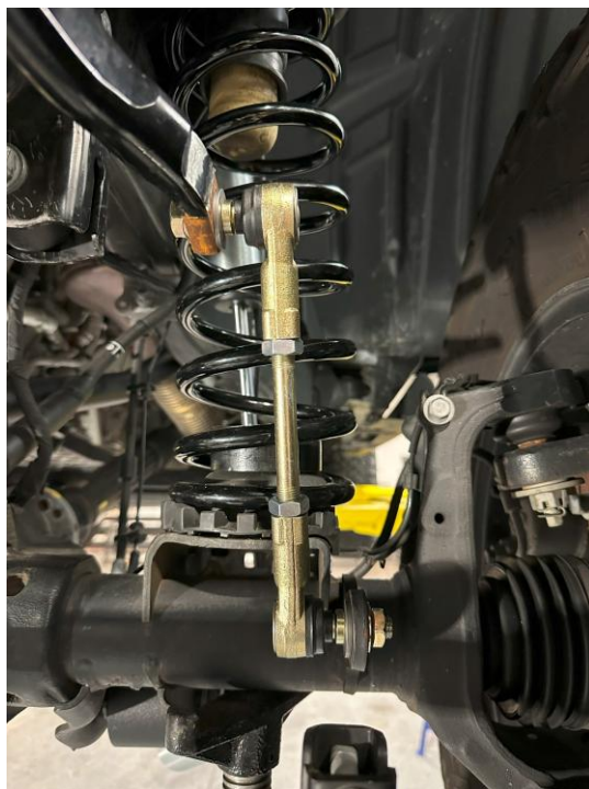
Figure 5: Sway bar end link on passenger side with proper conical washer orientation
