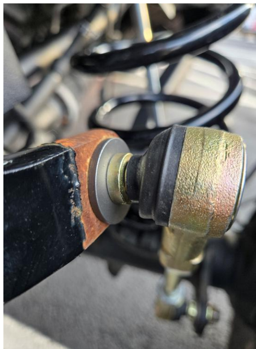
Figure 5: Sway bar end link on passenger side with proper conical washer orientation
