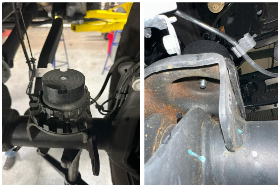
Figure 2: Bump stop installed on 2018+ JL axle
