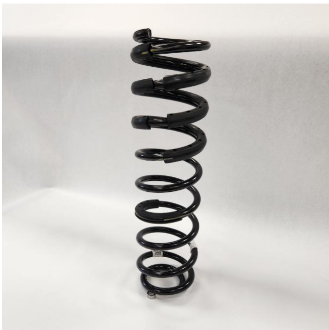
Figure 3: OEM coil with isolators
