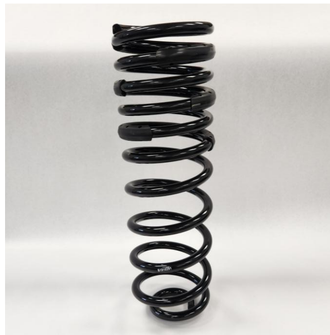
Figure 4: COR coil with isolators
