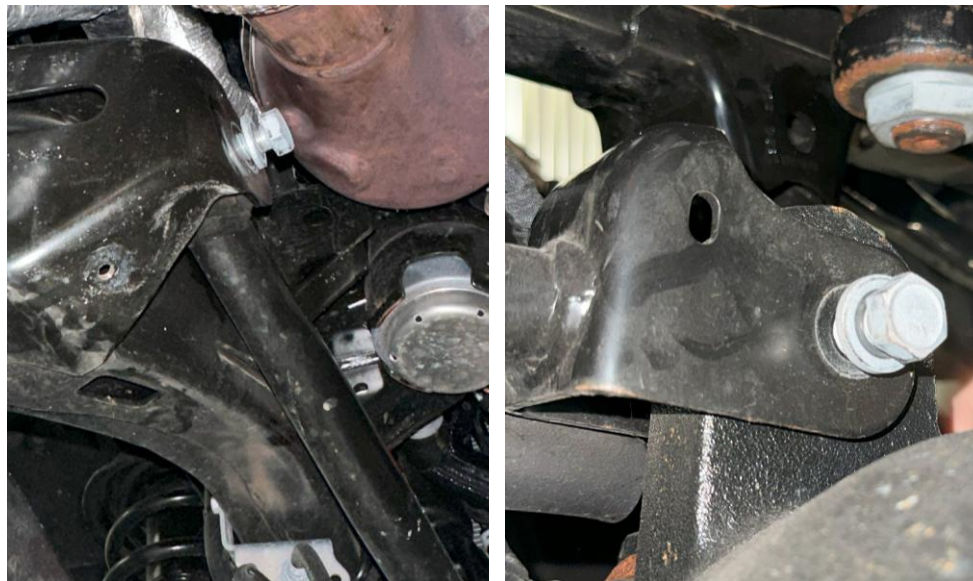
OEM Front upper control arm bolt frame and axle (driver-side)
