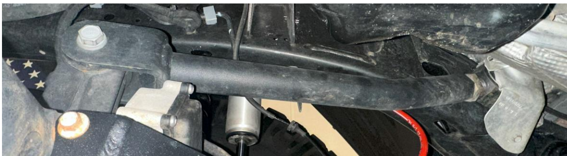
1709101 (OVERLAND+ Series) Front upper control arm installed
