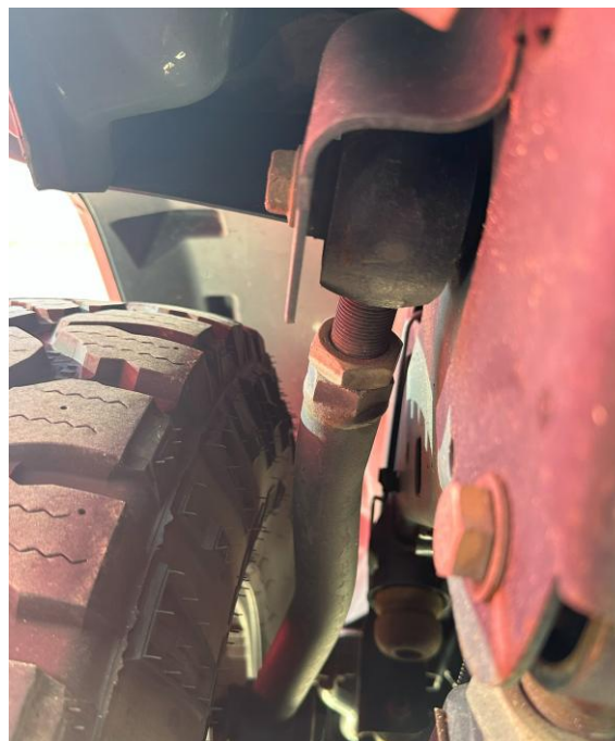
1709103 (OVERLAND+ Series) Rear upper control arm installed (JK 2-door)
