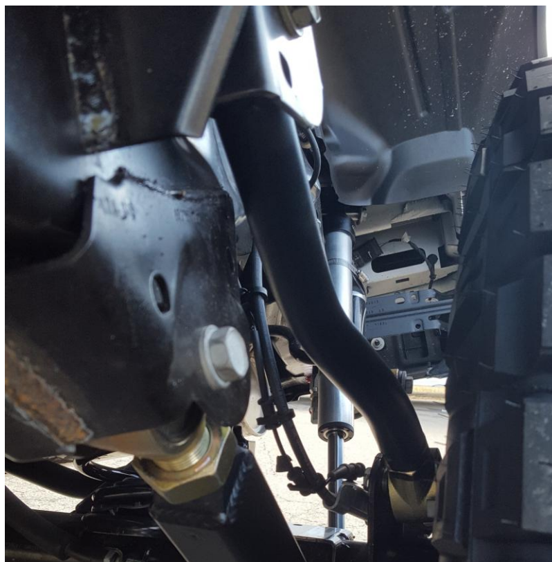
1709103 (PREMIUM Series) Rear upper control arm installed
