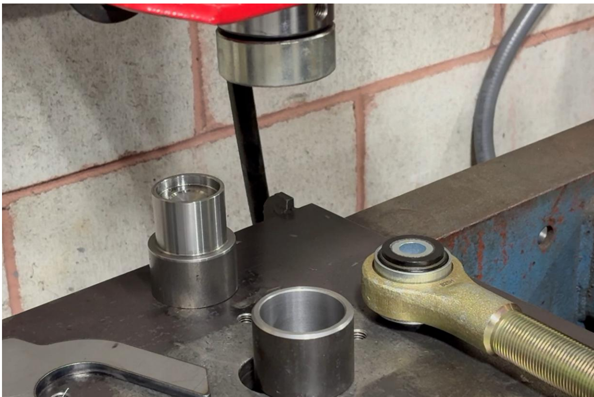
Figure 11: Bushing swap complete
