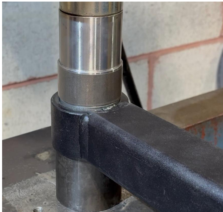
Figure 10: Sleeved end of the control arm with worn bushing pressed out and replaced
