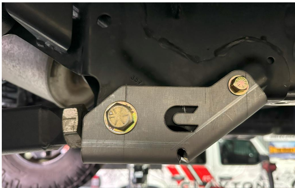
Figure 8: Prototype (unpainted) skid plate torqued to specification
