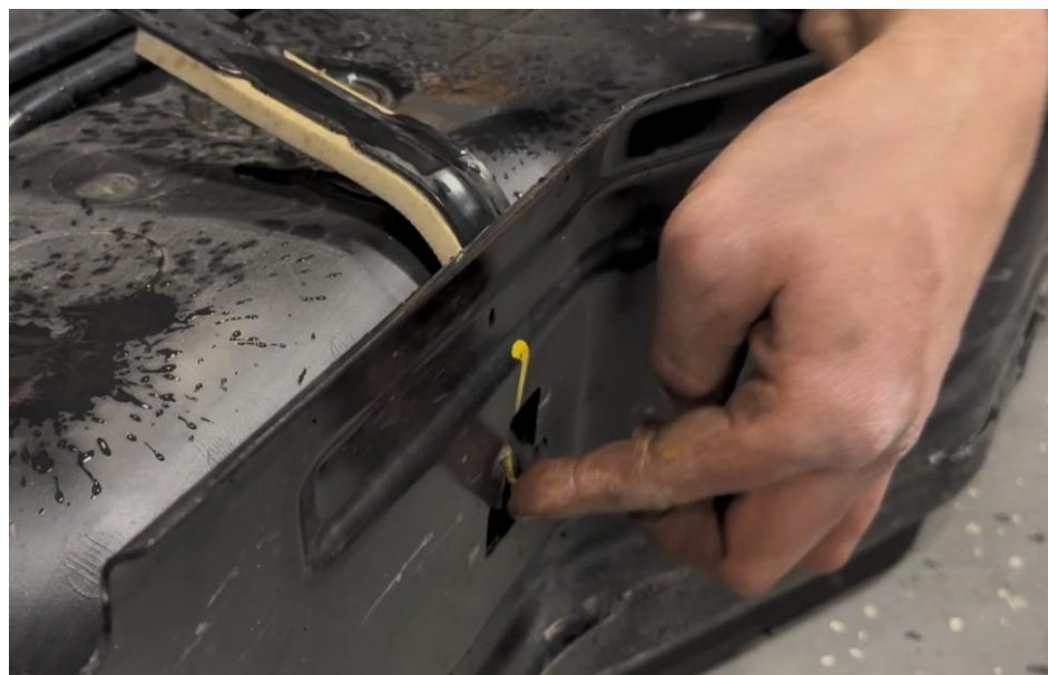
Figure 12: OEM tank strap removal
