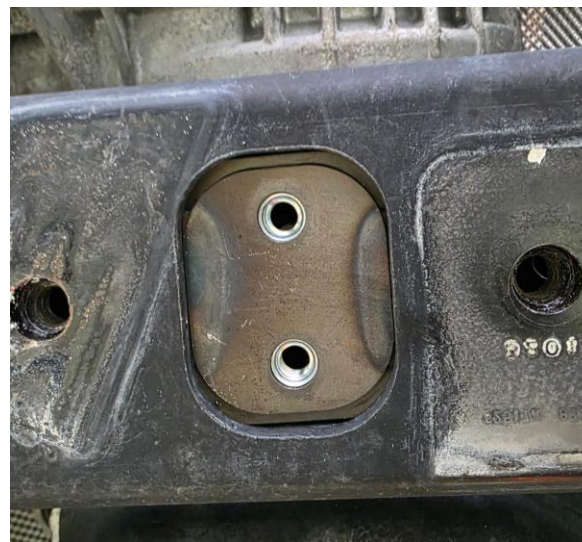
Figure 26: Installing cross-member components (Aluminum cross member)
