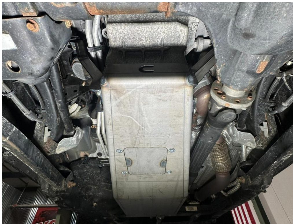
Figure 41: Engine skid plate fully installed
