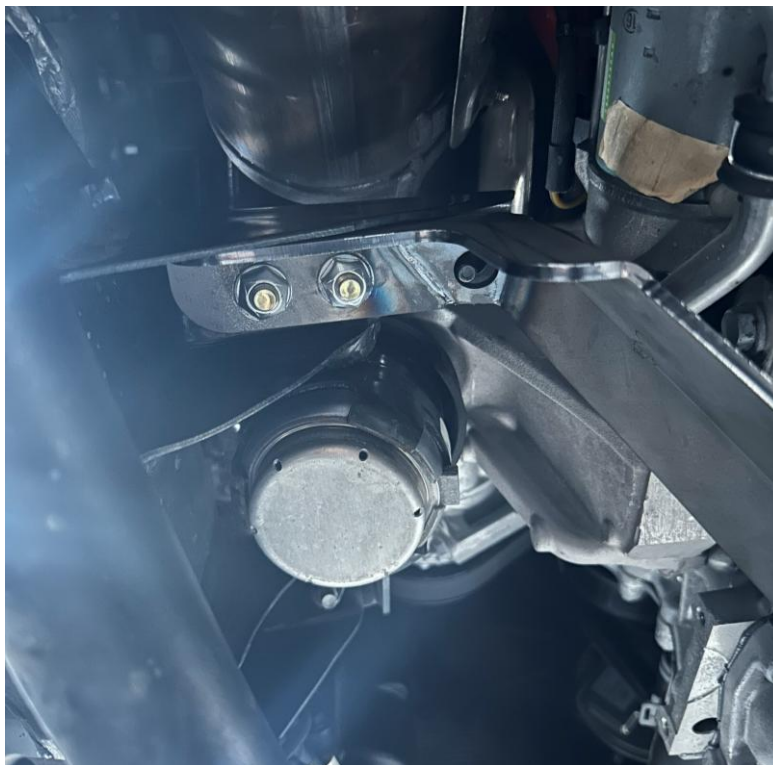
Figure 6: Motor mount bracket loosely installed
