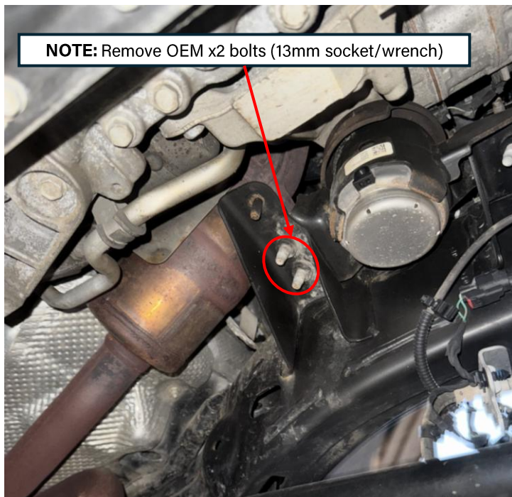
Figure 5: Motor mount old/new bolts with CAD visual showing bolt swap
