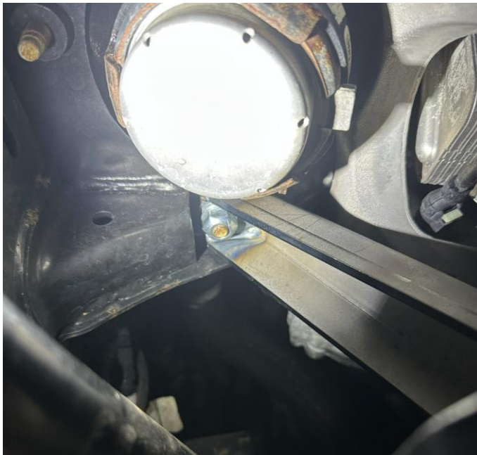
Figure 6: Motor mount bracket loosely installed
