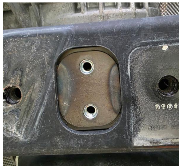
Figure 4: Installing cross-member components (Aluminum cross member)
