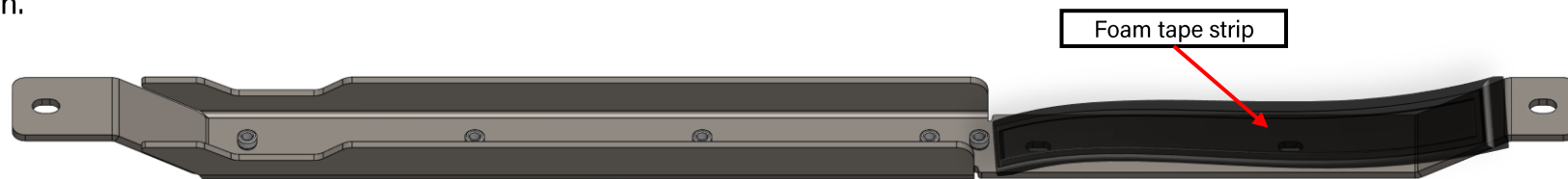
Figure 14: Skid support member with gasket tape applied
