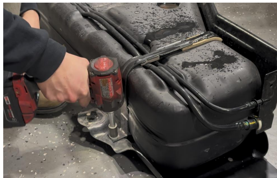
Figure 12: OEM tank strap removal
