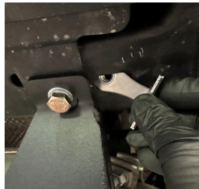
Figure 3: Teardrop flag nut install location
