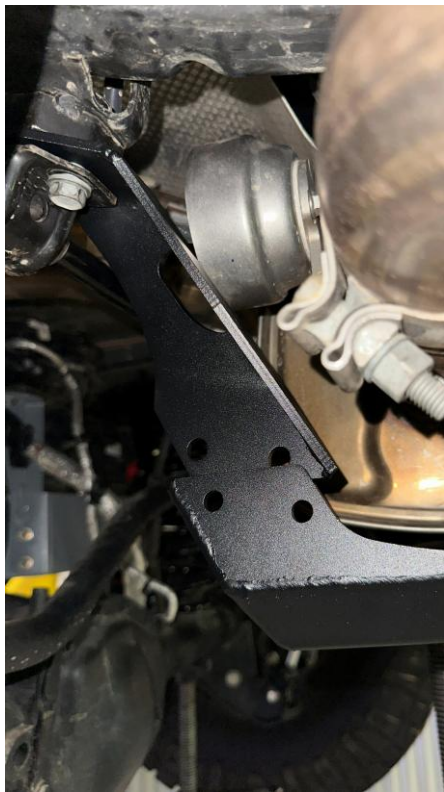
Figure 7: Driver's side rear support bracket loosely installed
