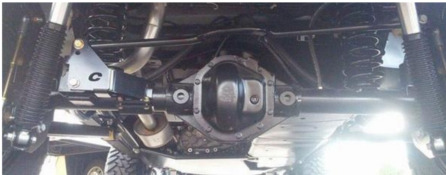
Jeep JK rear axle with new track bar relocation bracket installed
