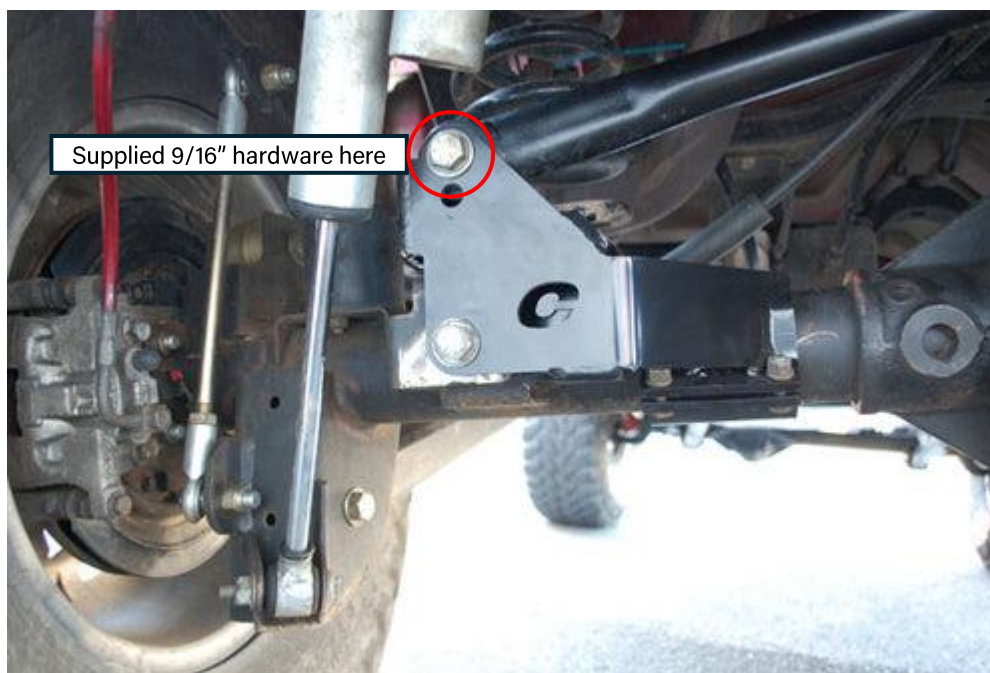
Jeep JK rear track bar relocation bracket new bolt installed
