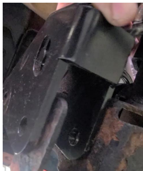
Positioning the rear track bar bracket around the original axle bracket
