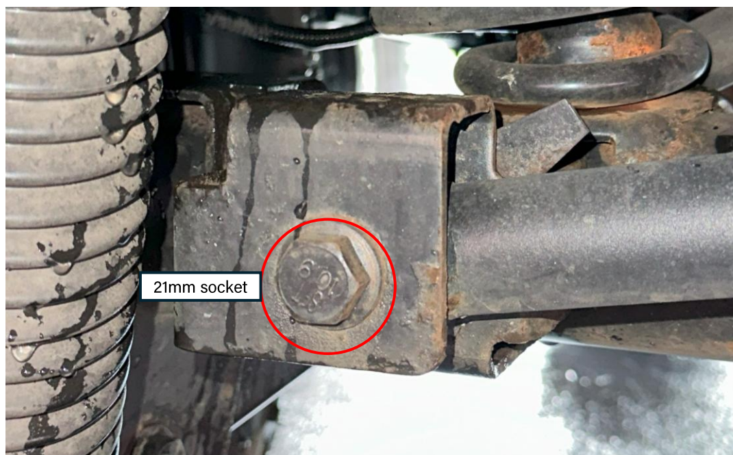
Jeep JK axle-side track bar bolt to be removed
