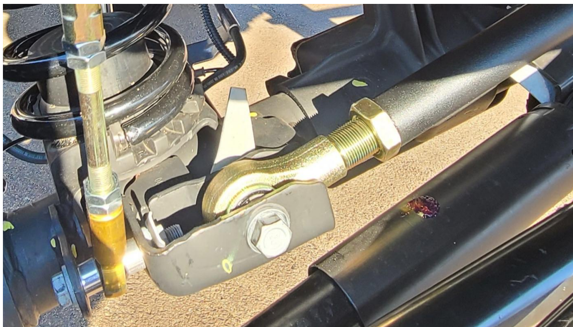
JL adjustable front track bar bolt installed hand-tight (axle-end)
