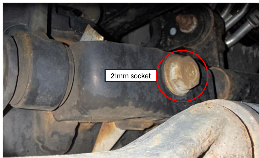
Jeep JL before and after axle-side track bar bolt is removed
