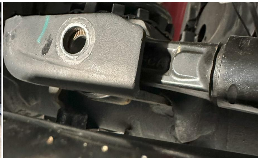
Jeep JL before and after axle-side track bar bolt is removed
