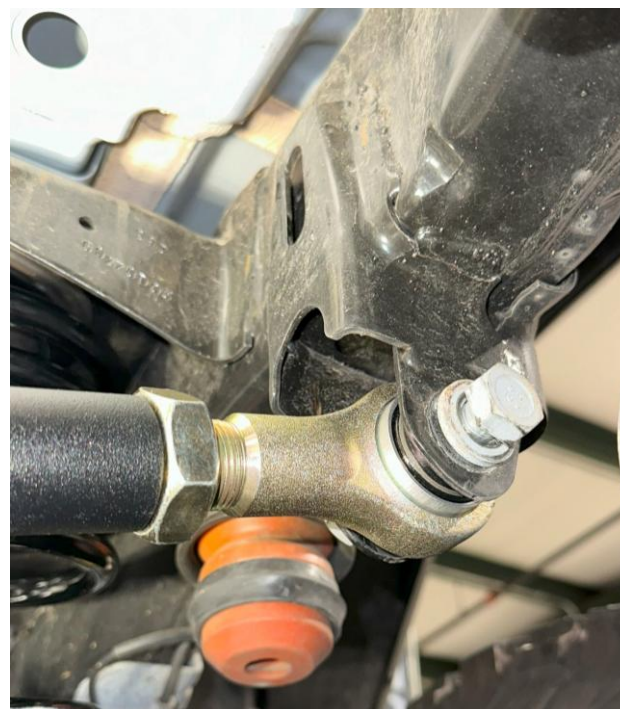
JL adjustable rear track bar before and after bolt install (hand-tight)
