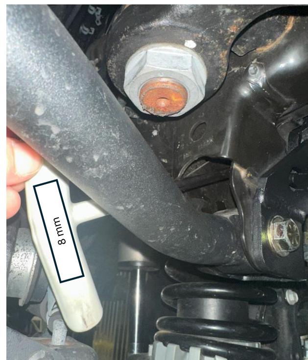
Figure 9: Tightening the remaining hex cap screw
