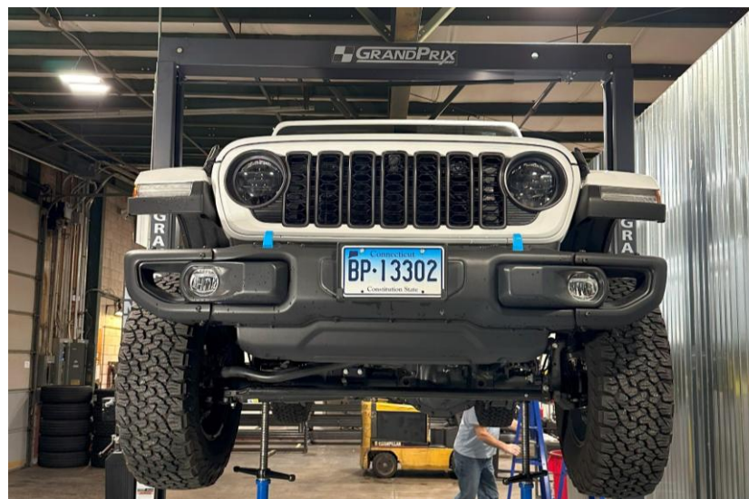
Figure 1: Vehicle positioned on two-post lift with supporting axle jack stands
