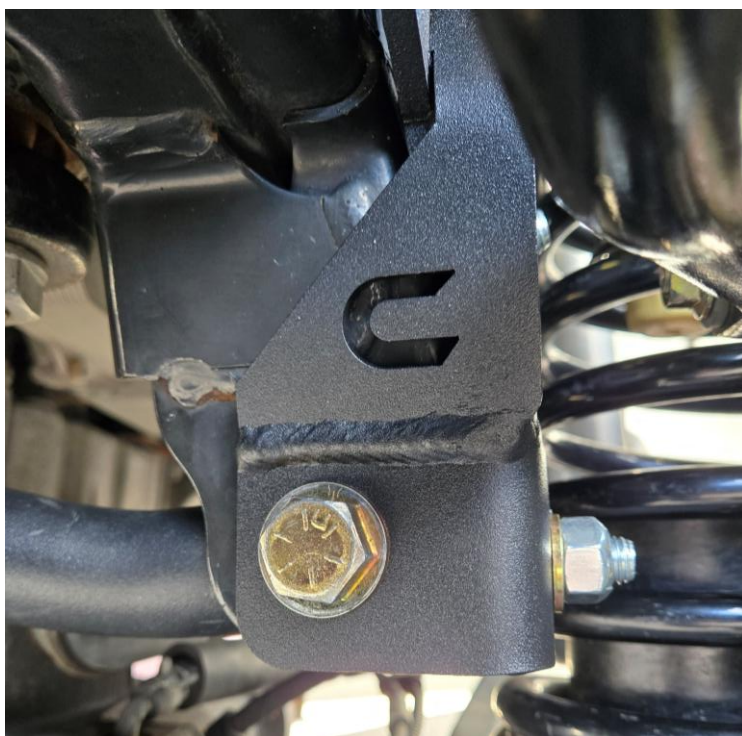
Figure 8: Torqued track bar bolt
