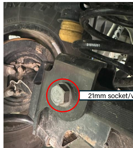
Jeep JT on four-post lift for installation and axle-side rear track bar bolt to be removed
