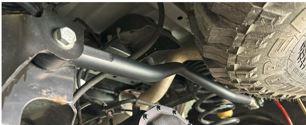
JT adjustable rear track bar bolt installed hand-tight (axle-end)
