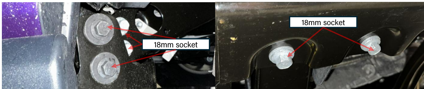
Figure B: 4x bolts near wheel well and 2x bolts on underside of frame
