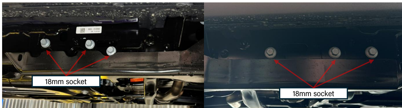
Figure A: passenger/driver side crash bracket bolts to remove (3x on each side)
