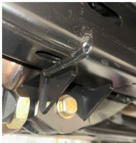
Figure 8: Bracket welded along edge to frame rail and area painted black
