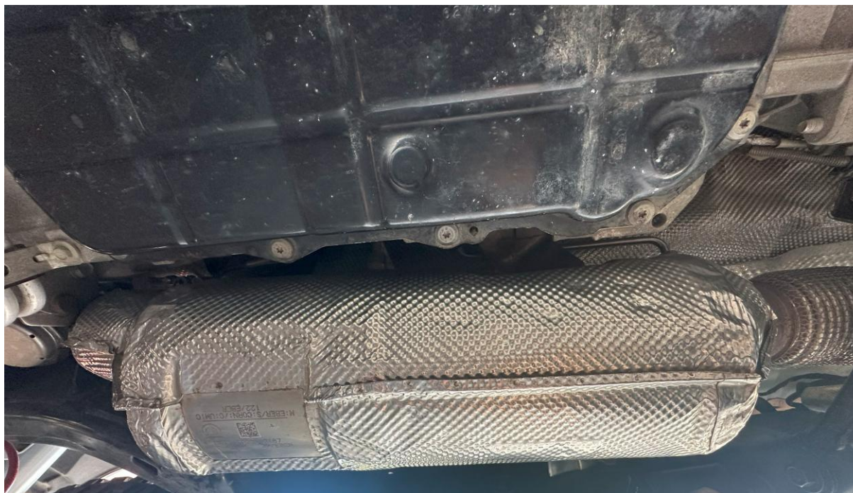
Figure 57: Catalytic converter reinstalled under the vehicle
