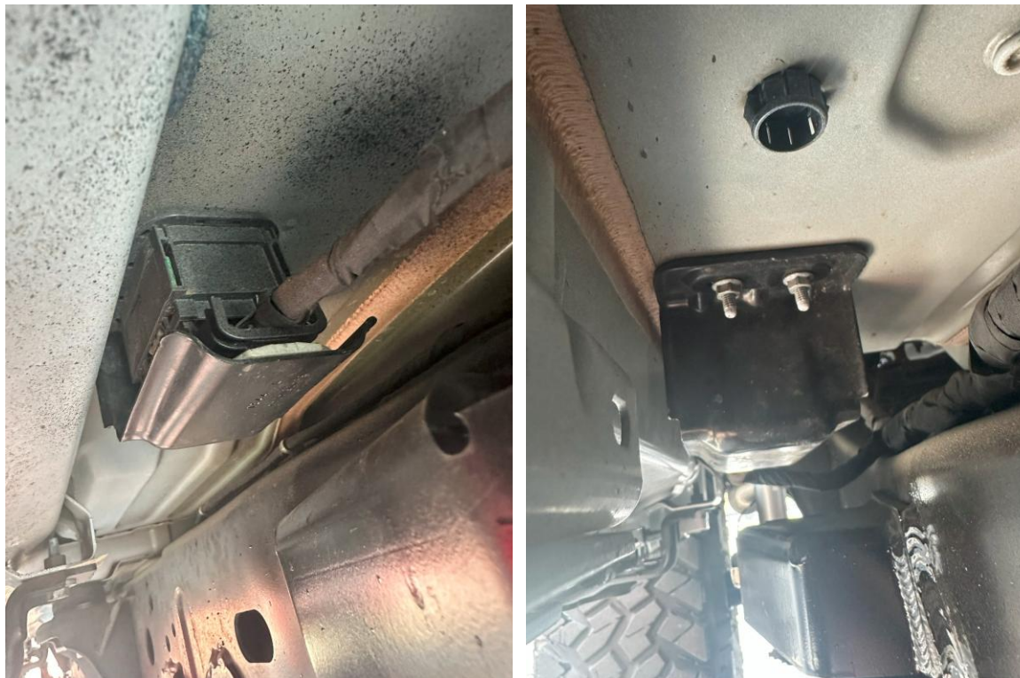
Figure 58: Wiring harness (both sides) reinstalled
