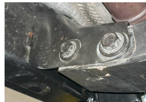
Figure 3: Cross-member bolts flipped around
