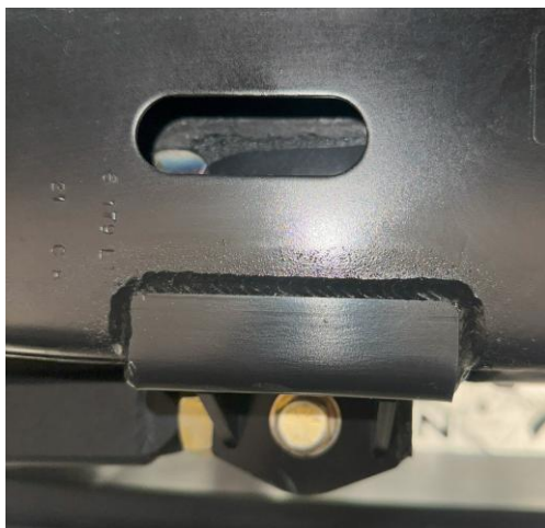
Figure 8: Bracket welded along edge to frame rail and area painted black
