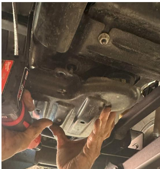
Figure 33: Removing x3 nuts at bottom plate
