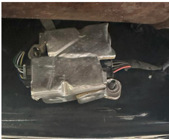
Figure 4j: Sensor to be removed off frame
