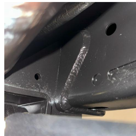
Figure 8: Bracket welded along edge to frame rail and area painted black
