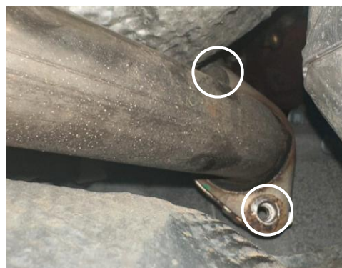
Figure 4c: Flange to be removed (x2 bolts)
