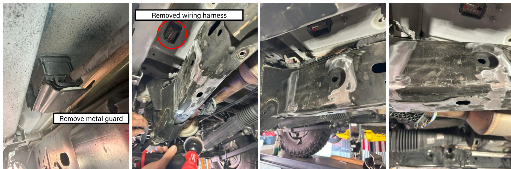
Figure 44: Frame rails prepped for bracket positioning
