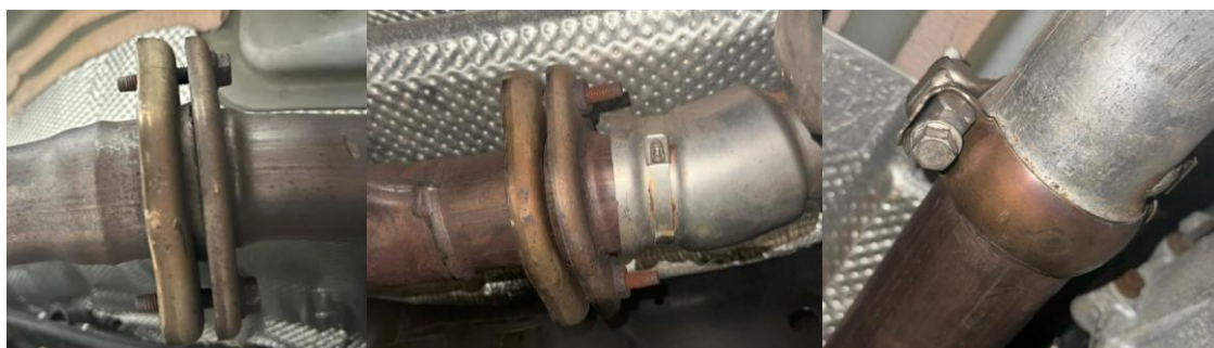
Figure 4: Exhaust section flanges and clamps
