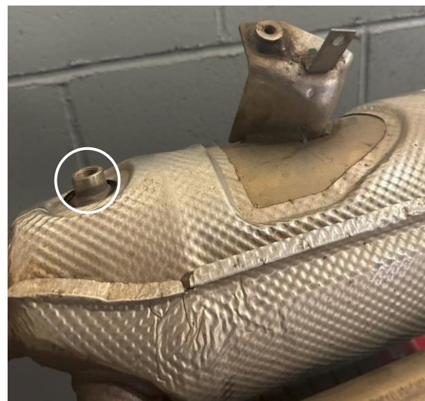
Figure 4i: x1 port at rear of section
