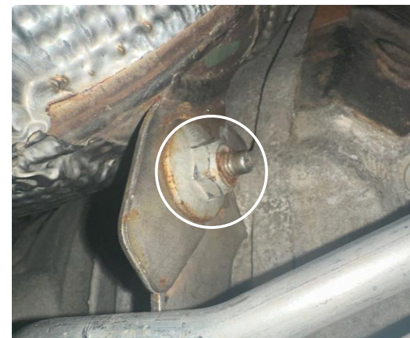
Figure 4g: Hanger nut to be removed
