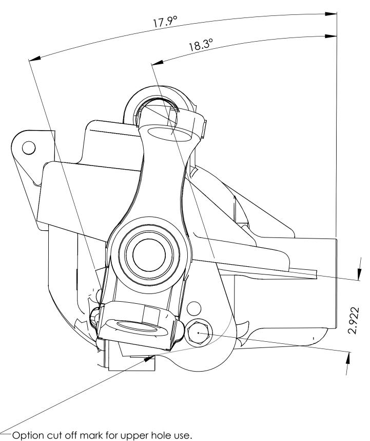
This is an optional hole which moves the lower control arm mount up 1". Using this hole may cause changes in handling and add more stress to the upper control arms.
