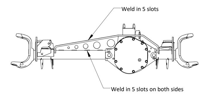
Step 10: Weld 2 posts into cut outs.
