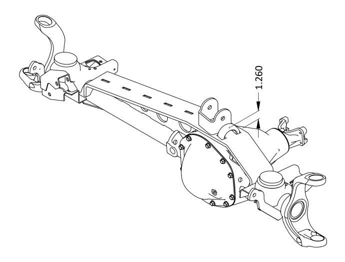
Step 8: Make 5 welds in slots to gusset and axle tube on both sides.
