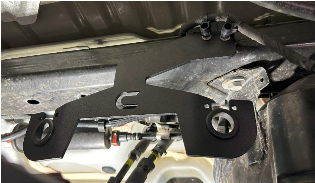
Figure 5: Installed bracket with proper bend direction
