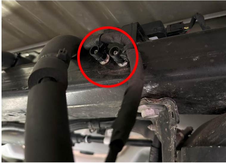
Figure 4: 10mm nuts to be removed to mount bracket
