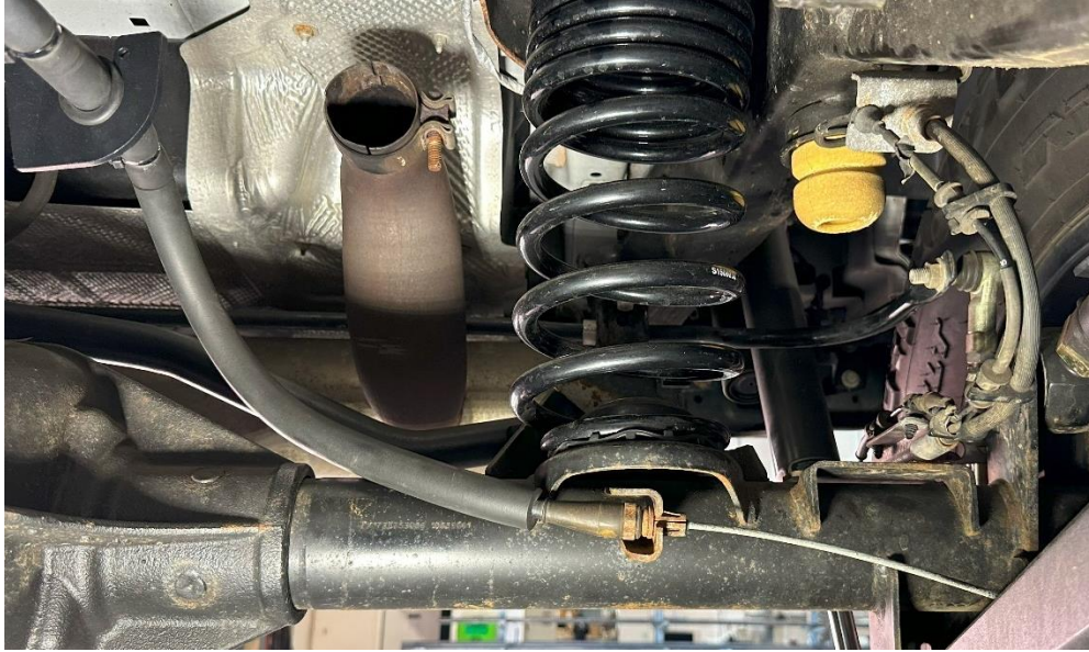
Figure 8: Right side emergency brake cable housing installed in axle bracket
