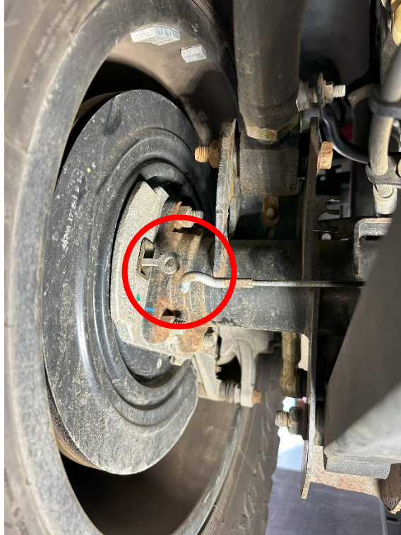
Figure 1: Left rear emergency brake cable removed from eyelet
