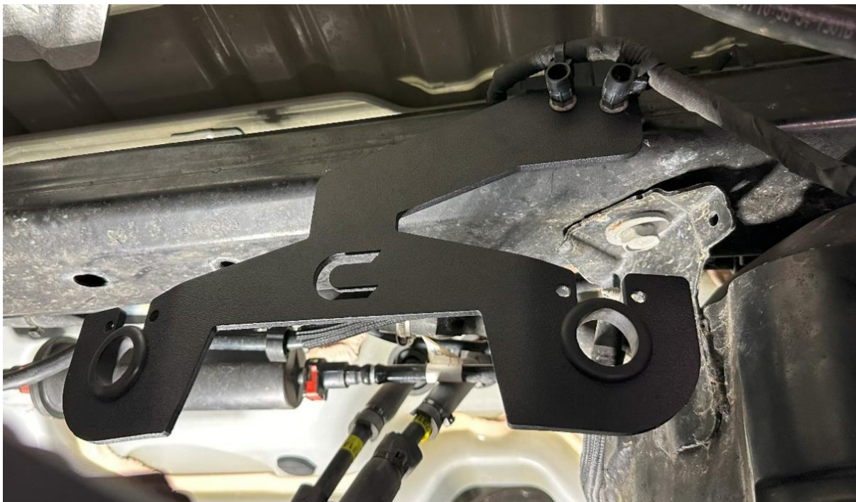
Figure 6: Bracket installed with proper orientation, and 10mm nuts tightened
