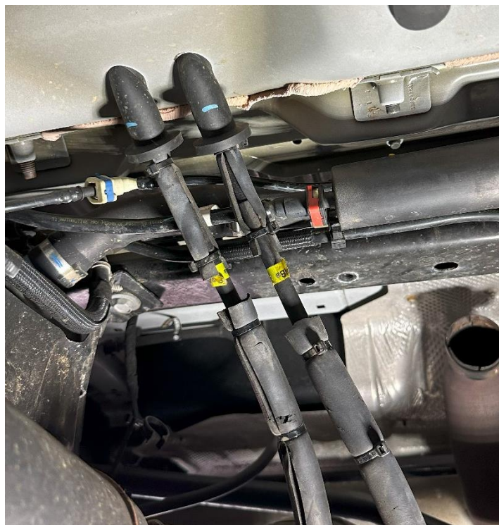
Figure 4: Parking brake cable housings pulled out from above the cross member and rerouted below the fuel line
