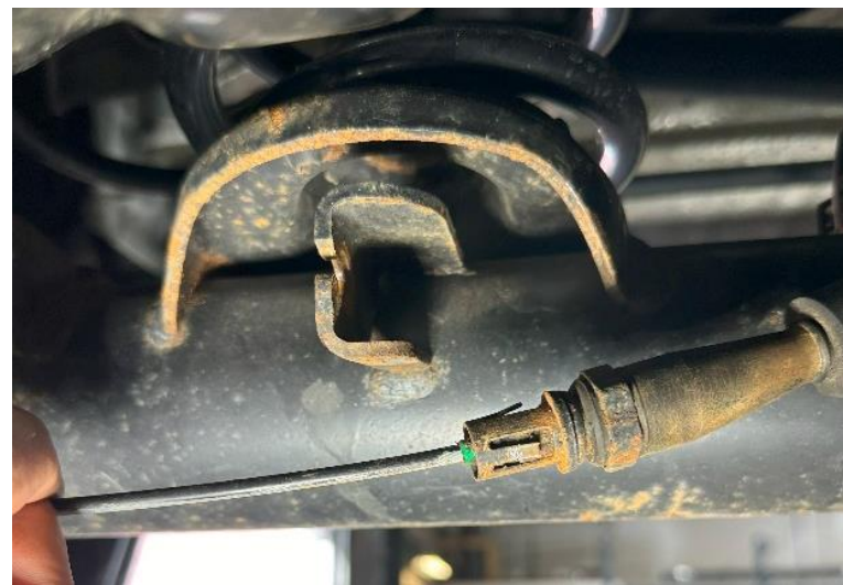
Figure 2: Emergency brake cable housing spring clips fully compressed
