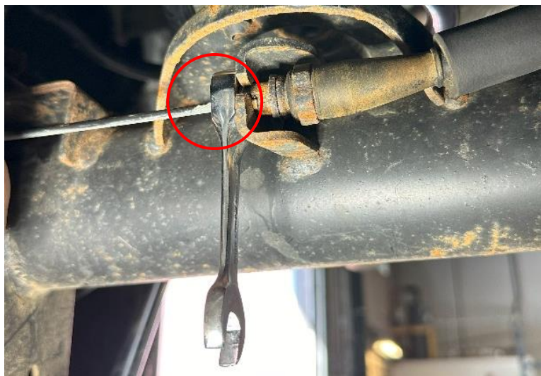
Figure 2: Emergency brake cable housing spring clips fully compressed
