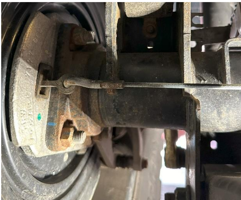
Figure 10: Rear left cable reinstalled in eyelet hook
