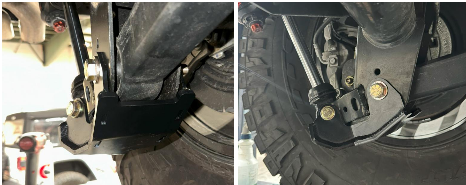
Figure 7: Skid plate torqued to specification
