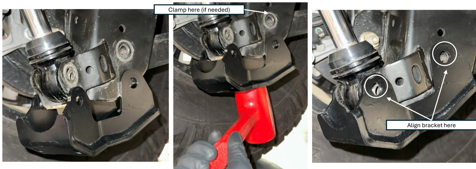
Figure 3: Left skid plate bracket fitting process
