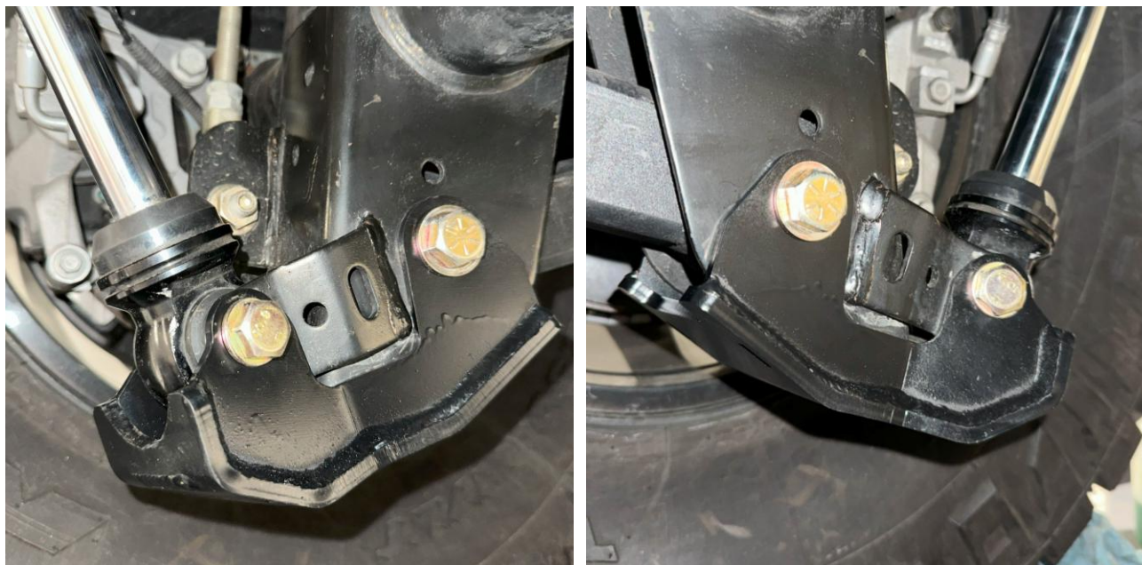
Figure 6: Left and right bracket installed
