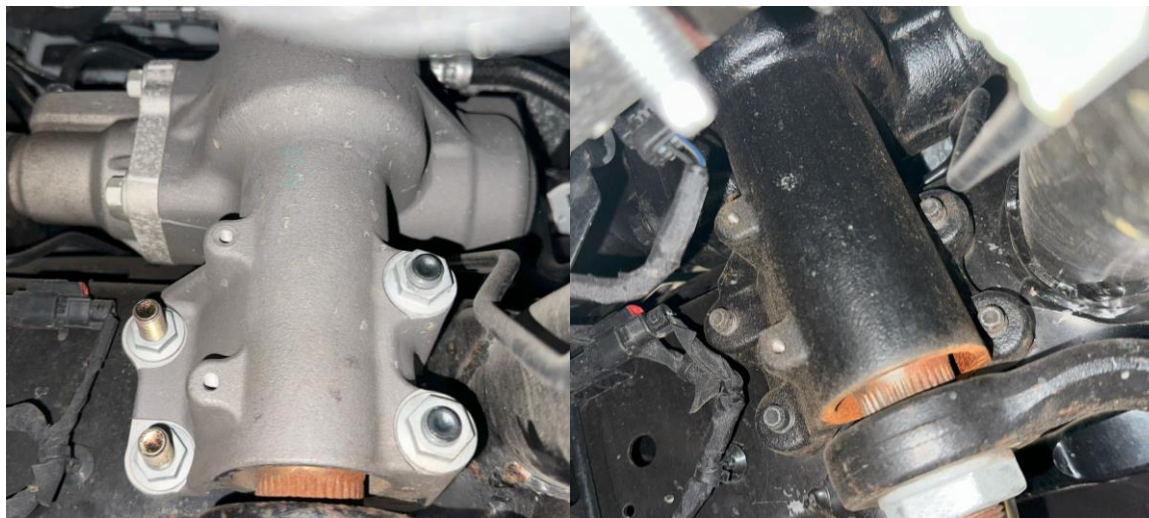
Figure 4: Aluminum steering box (left) vs. steel steering box (right)
