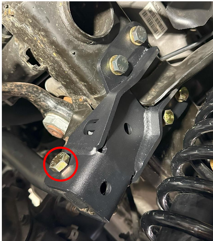
Figure 5: Steering box bolts installed with temporary track bar bolt installed
