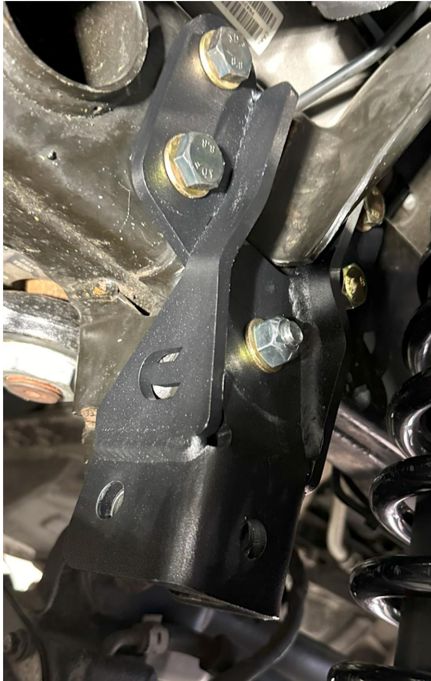
Figure 6: Removed track bar bolt after installing and tightening the top hex drive bolt
