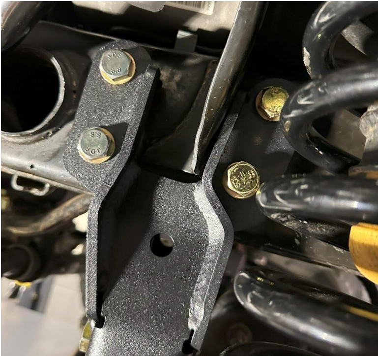
Figure 3: 4 steering box bolts installed (tighten, do not torque)
