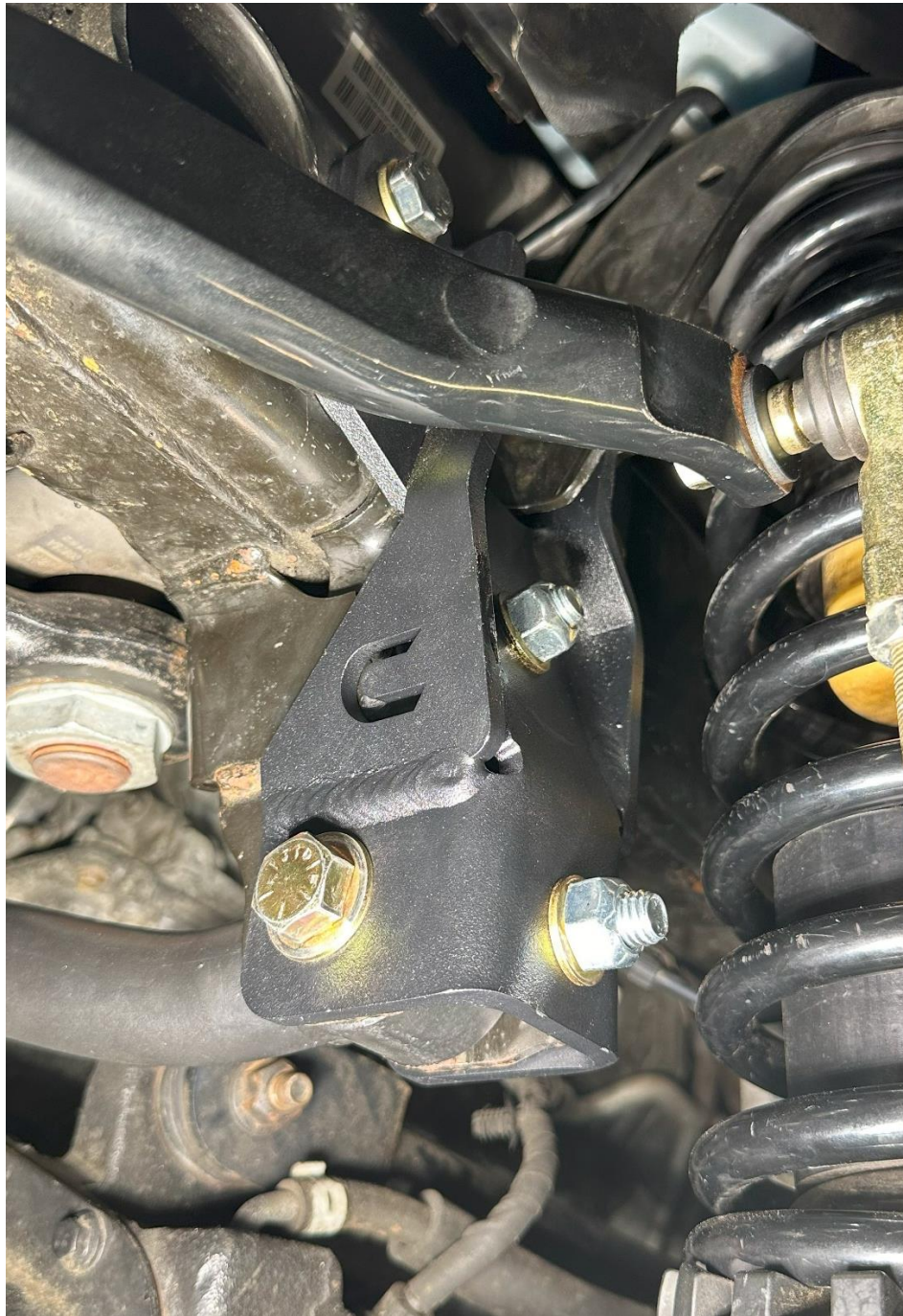
Figure 8: Track Bar Reinforcement Bracket installed
