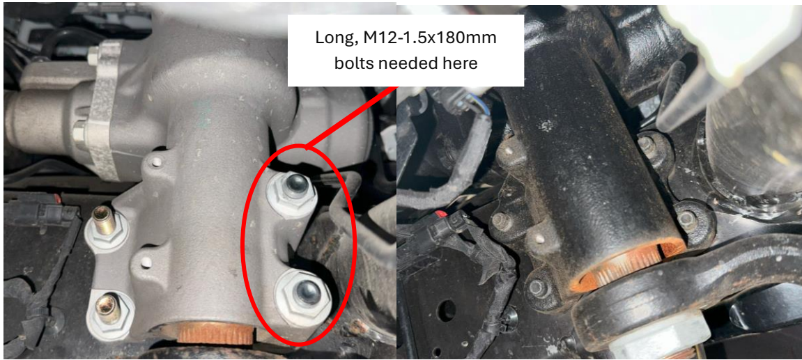
Figure 4: Aluminum steering box (left) and steel steering box (right)
