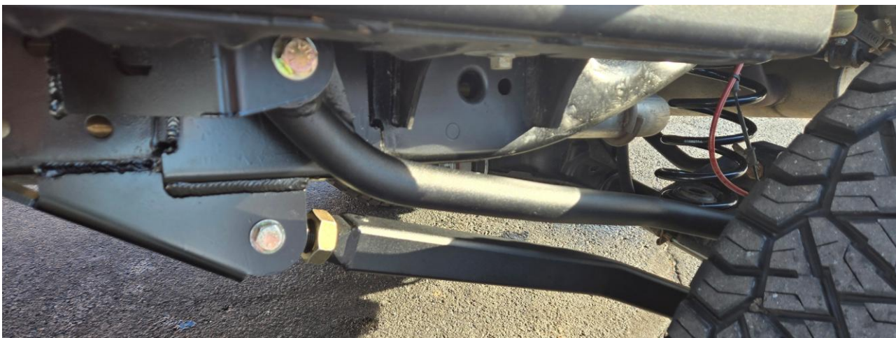
Figure 19: Driver side lower and upper control arms installed
