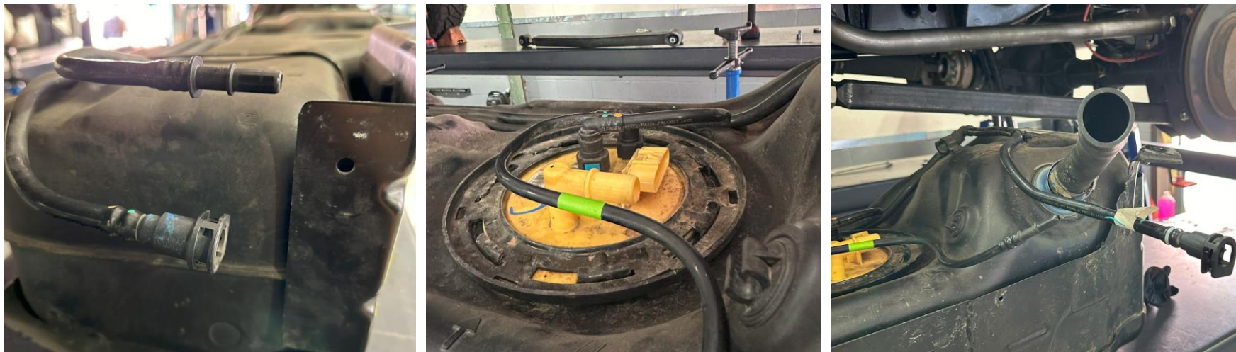
Figure 23: Front, top and rear fuel tank connections
