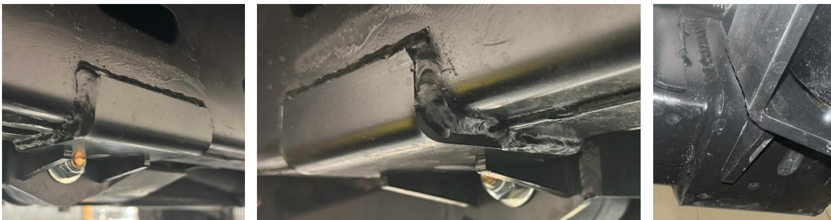
Figure 8: Bracket welded along edge to frame rail and area painted black
