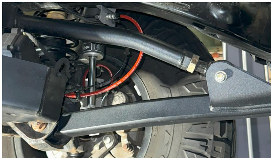
Figure 10: Passenger side lower and upper control arms installed
