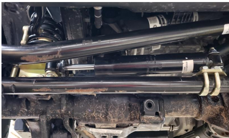
Figure 7: Factory steering stabilizer (left) and Fox steering stabilizer (right) installed with COR-5209010 Tie Rod Clamp on Jeep JL
