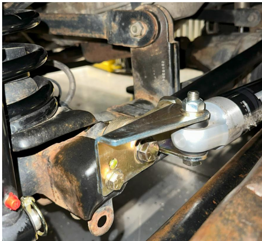
Figure 8: Stock steering stabilizer and fox steering stabilizer installed with COR- 5200940, Tie Rod Clamp
