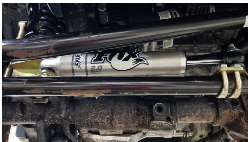
Figure 7: Factory steering stabilizer (left) and Fox steering stabilizer (right) installed with COR-5209010 Tie Rod Clamp on Jeep JL
