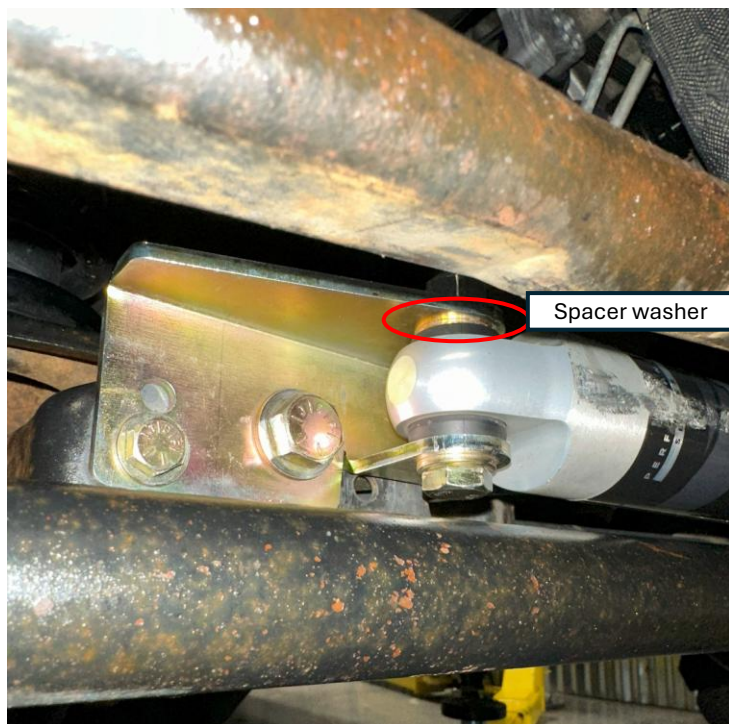
Figure 6: Steering stabilizer installed with the bolt head on the bottom of the bracket, and spacer washer installed
