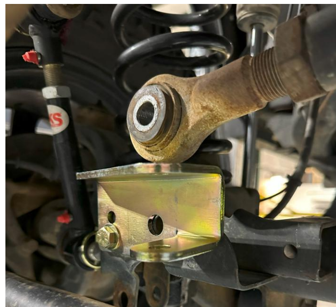
Figure 4: 3/8" bolt with washer, lock washer, and nut installed, with track bar bolt hole aligned
