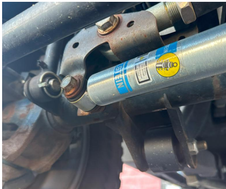
Figure 2: Factory steering stabilizer axle mount location
