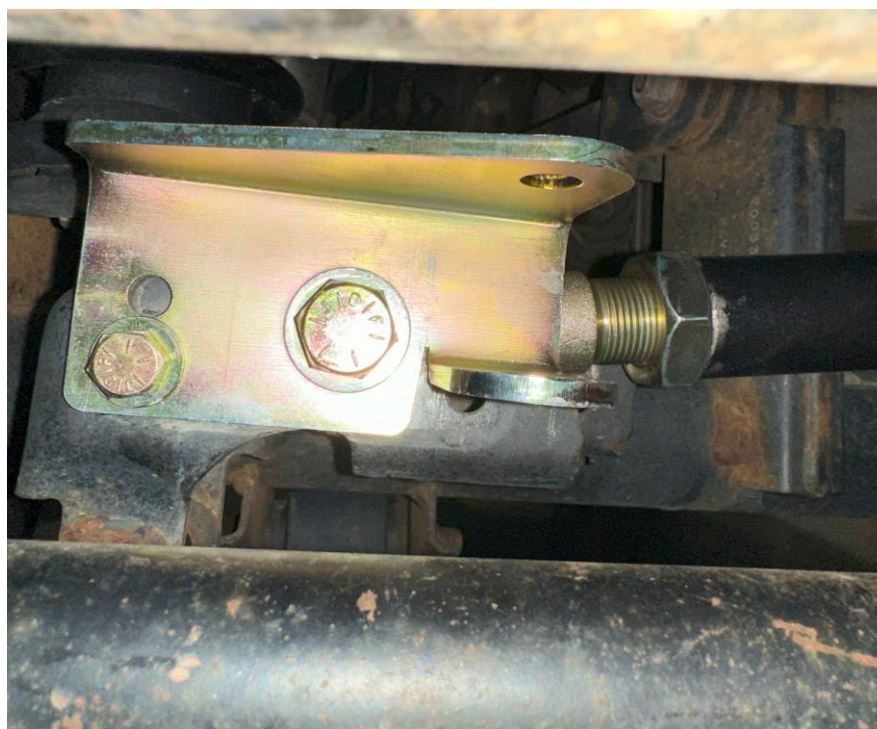
Figure 5: Track bar reinstalled with included 9/16" bolt, washers, and lock tab
