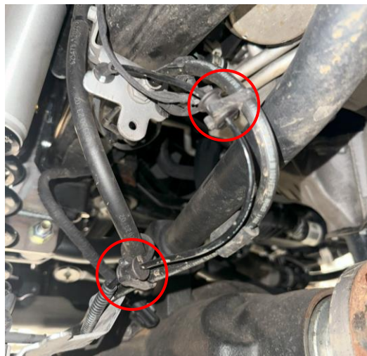
Old brake-line clips to be removed
