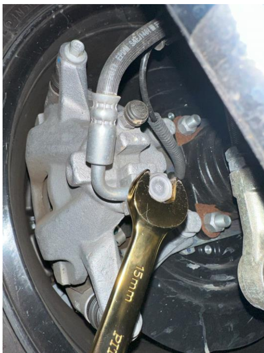
Brake caliper banjo bolt (15mm)
