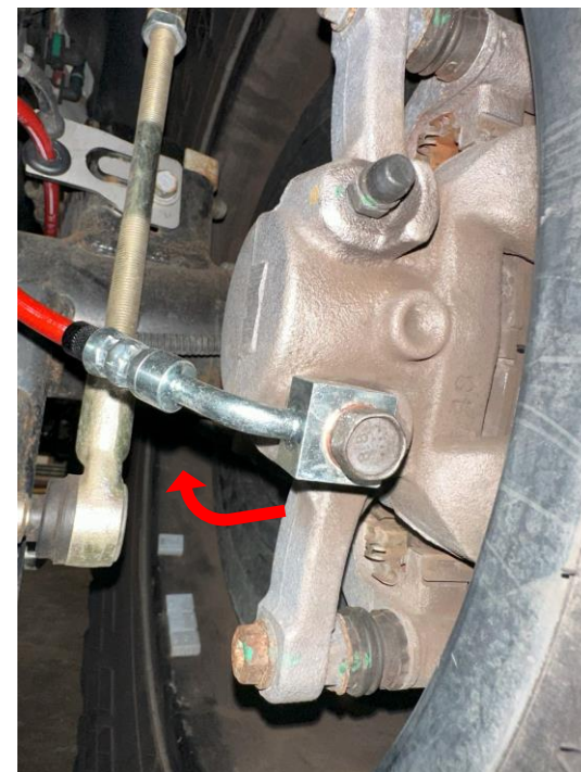
New banjo fitting installed (rear passenger's side)
