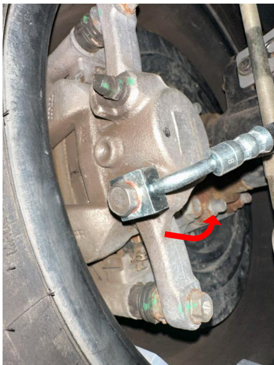
New banjo fitting installed (rear driver's side)
