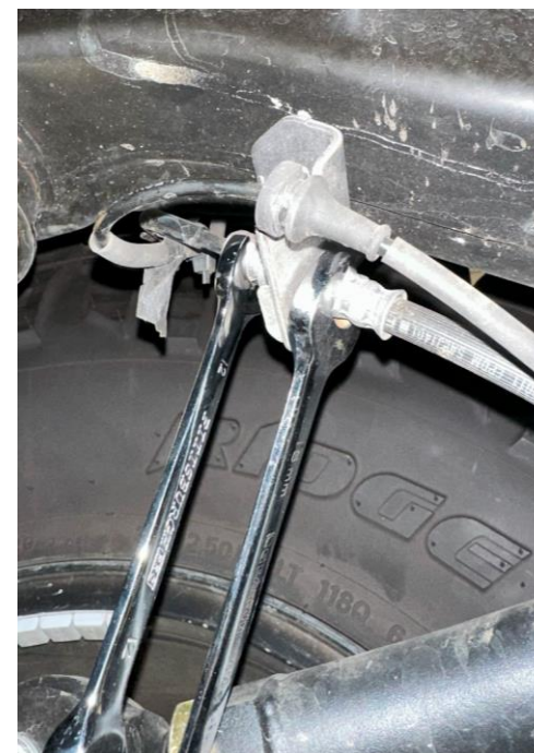
Frame end fitting (16mm and 12mm)
