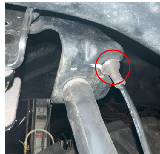
Frame mount ABS cable to be removed
