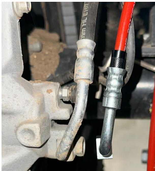
Proper Banjo Fitting orientation (rear driver's side)
