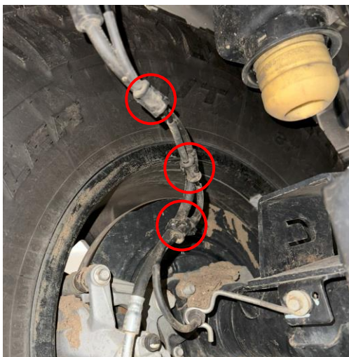
Old brake-line clips to be removed
