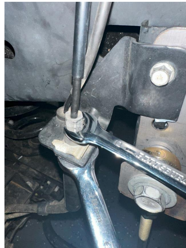
Frame end fitting (16mm and 12mm)
