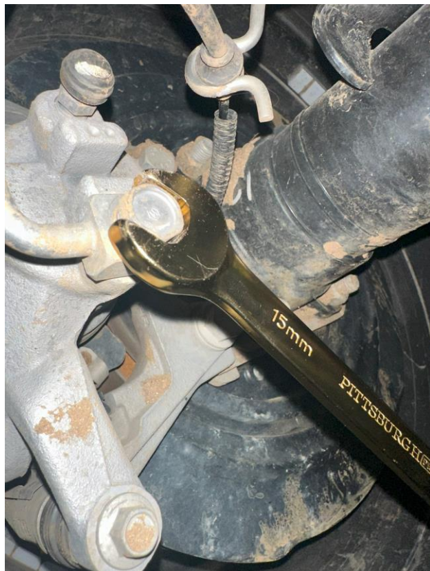
Brake caliper banjo bolt (15mm)
