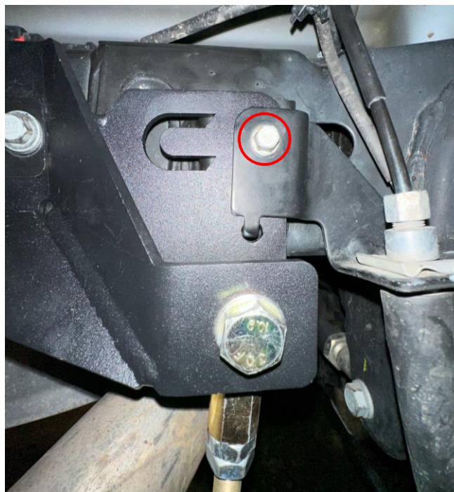
Figure 5: Brake line bracket mounted over “C” wedge plate
