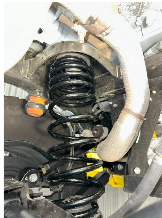
Figure 30: New rear springs installed and seated properly
