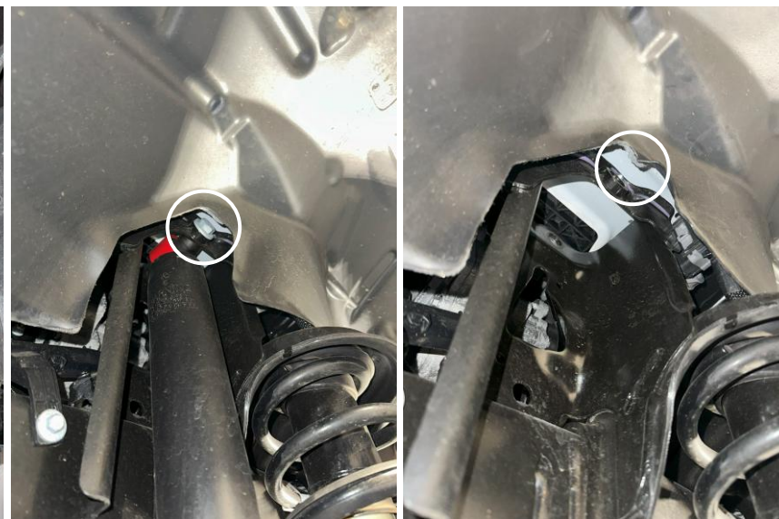
Figure 5: Front upper passenger shock bolt removed
