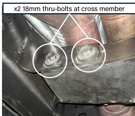
Figure 11d: Cross-member bolts
