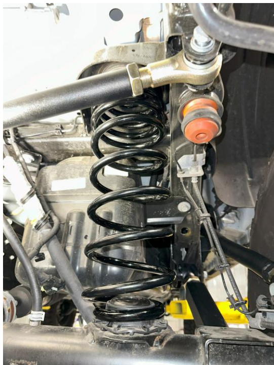
Figure 30: New rear springs installed and seated properly
