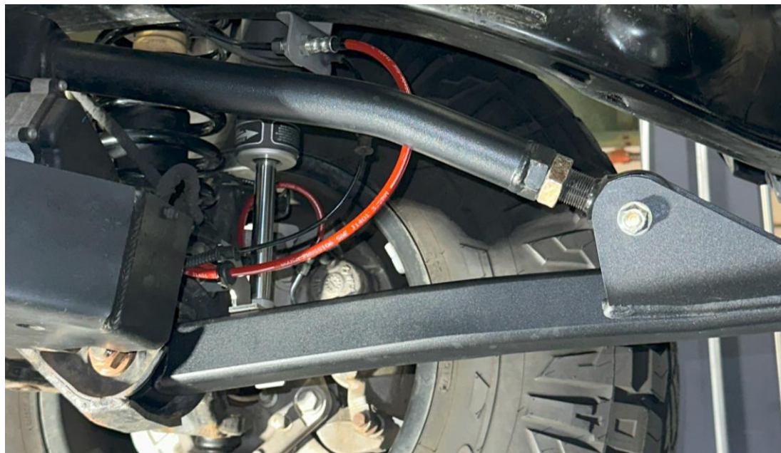
Figure 18: Front long arm kit installed
