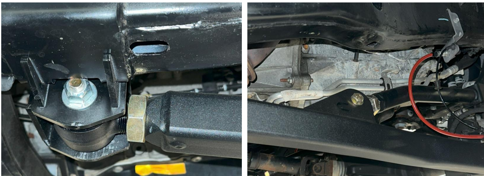
Figure 12: Front frame brackets and long arms installed
