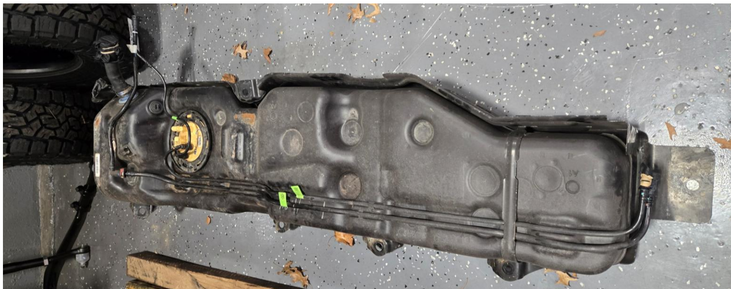
Figure 27: Gas tank dropped (follow instructions from COR-5009200/4809200/5009300/4809300)
