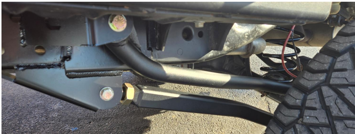
Figure 28: Rear frame brackets and long arms installed
