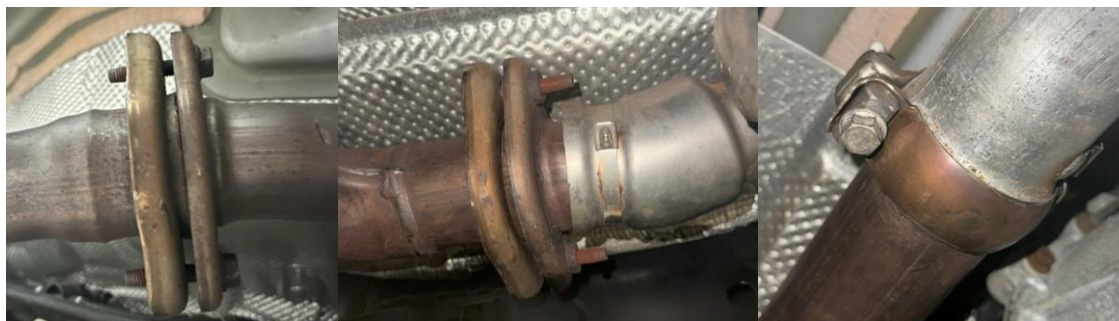
Figure 4: Exhaust section flanges and clamps
