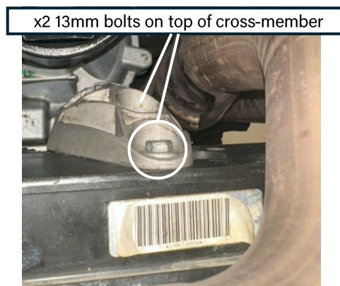
Figure 4c: Cross-member exhaust hanger
