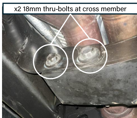
Figure 4d: Cross-member bolts
