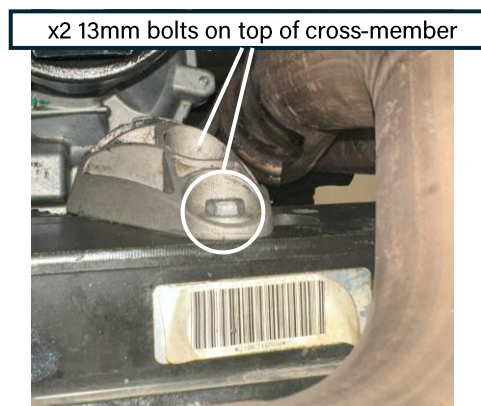
Figure 4c: Cross-member exhaust hanger
