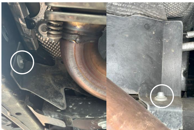
Figure 13: Fuel-line shield bolts (passenger side)
