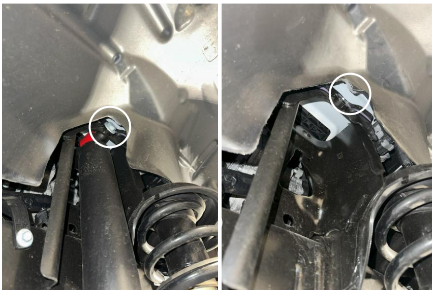
Figure 5: Upper passenger shock bolt removed
