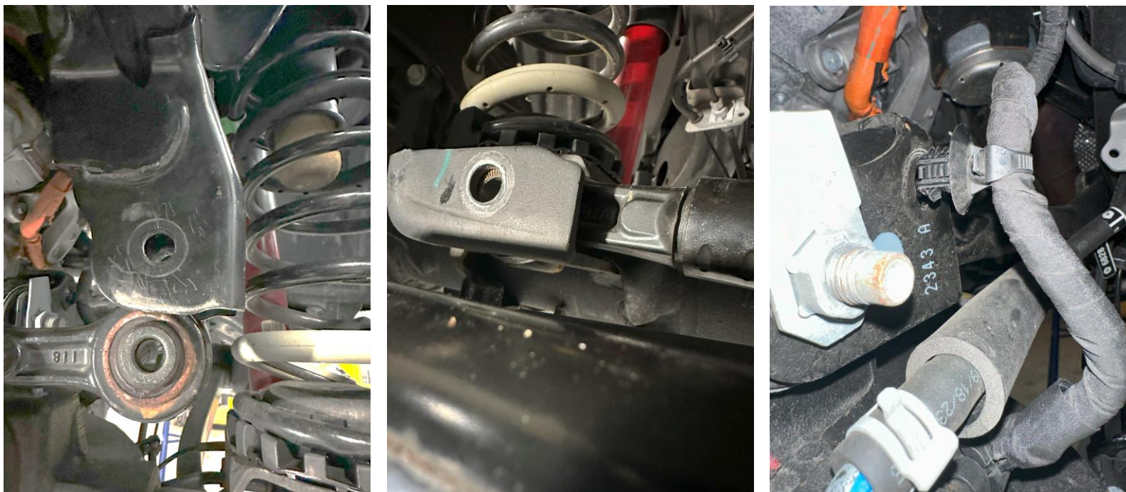
Figure 3: Front factory track bar bolt at frame and axle removed, with differential sensor clip removed
