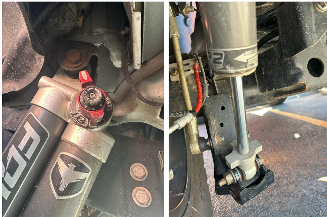
Figure 31: Rear shock top and bottom bolt installed loosely
