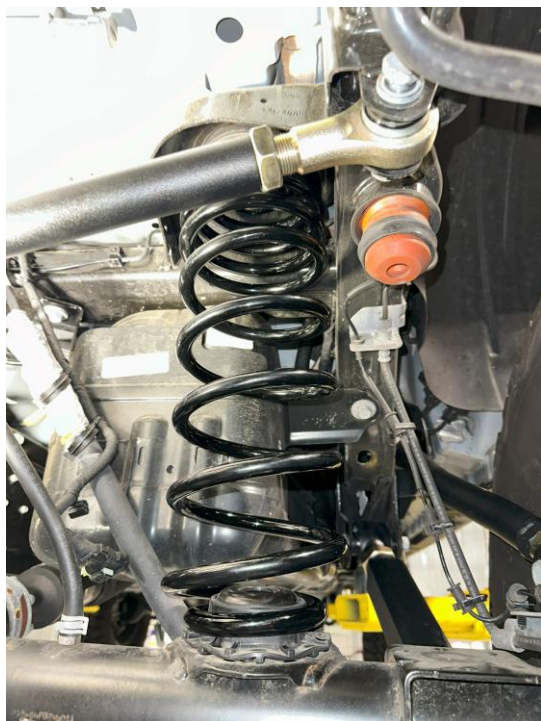
Figure 29: New rear springs installed and seated properly
